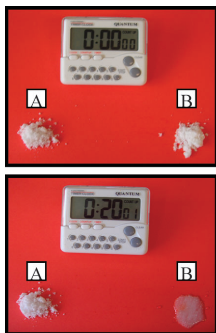
Fig. 6 The effect of moist air on hydrophobic EMIM triflimide (sample A) and hydrophilic EMIM Br (sample B). After 20 min exposure to normal air at room temperature the EMIM Br has absorbed enough moisture from the atmosphere to turn from a solid into a liquid.
