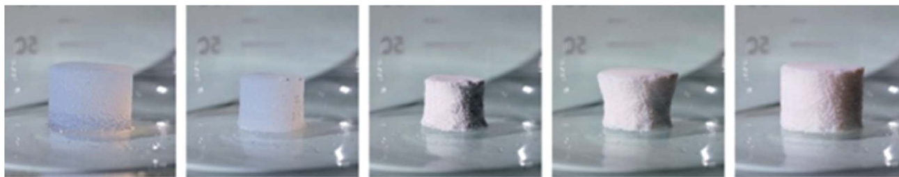
Fig. 3 Silica aerogel composites synthesised with polymethylsilsesquioxane precursors and dispersed boehmite nanofibres, under ambient pressure drying conditions: a temporal shrinkage followed by re-expansion can be observed, due to the spring-back effect (reprinted with permission from ref. 138. Copyright 2016, American Chemical Society).
