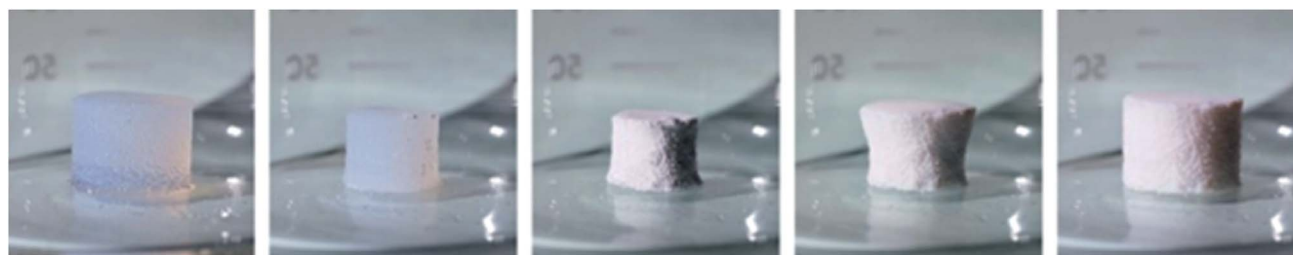
Fig. 3 Silica aerogel composites synthesised with polymethylsilsequioxane precursors and dispersed boehmite nanofibres, under ambient pressure drying conditions: a temporal shrinkage followed by re-expansion can be observed, due to the spring-back effect (reprinted with permission from ref. 138. Copyright 2016, American Chemical Society).
