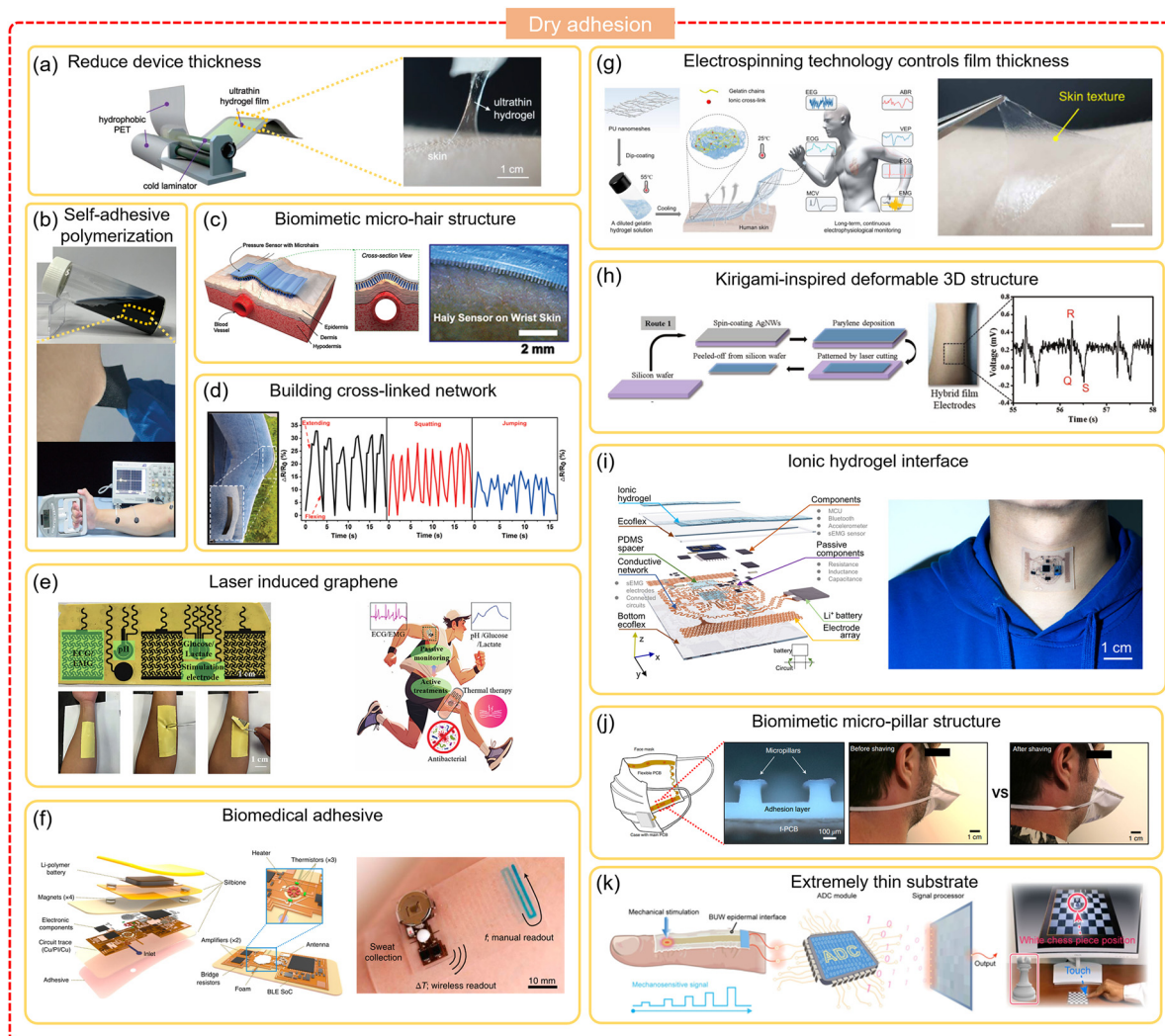
Fig. 8 Schematic diagrams illustrating the application of dry adhesion in flexible electronics. (a) Ultra-thin hydrogel films suitable for skin-integrated electronics. Adapted with permission under a Creative Commons CC BY License from ref. 167. Copyright 2022 The Authors, published by John Wiley and Sons. (b) Self-adhesive ink for monitoring EMG signal on the skin. Adapted with permission under a Creative Commons Attribution 4.0 International License from ref. 171. Copyright 2022 The Authors, published by Springer Nature. (c) Pressure sensors with microhair structures for highly conformal skin contact and pulse detection. Reproduced with permission from ref. 101. Copyright 2014, John Wiley and Sons. (d) Sensors mounted on the knees to monitor the corresponding signals of flexion, squatting, and jumping. Reproduced with permission from ref. 172. Copyright 2021, John Wiley and Sons. (e) The thickness of the device is reduced by means of laser induced graphene for monitoring ECG signal. Adapted with permission under a Creative Commons CC BY License from ref. 173. Copyright 2024 The Authors, published by John Wiley and Sons. (f) Build a skin interface platform with biomedical adhesives for monitoring biochemical information. Adapted with permission under a Creative Commons CC BY License from ref. 174. Copyright 2021 The Authors, published by Springer Nature. (g) ECG signal monitoring is realized by controlling material thickness by means of electrospinning. Reproduced under terms of the Creative Commons Attribution 4.0 International License from ref. 175. Copyright 2024 The Authors, published by American Association for the Advancement of Science. (h) Inspired by kirigami, a 2D flat surface is transformed into a 3D surface for monitoring EMG signal. Adapted with permission under a Creative Commons CC BY License from ref. 176. Copyright 2018 The Authors, published by John Wiley and Sons. (i) The ionic hydrogel interface was constructed to monitor physiological signals. Adapted with permission under a Creative Commons Attribution 4.0 International License from ref. 177. Copyright 2023 The Authors, published by Springer Nature. (j) Comfortable electronic devices attached to face mask for collecting environmental and biological data. Adapted with permission under a Creative Commons CC BY License from ref. 69. Copyright 2022 The Authors, published by Springer Nature. (k) HMI device is used to control the position movement of chess pieces. Adapted with permission under a Creative Commons CC BY License from ref. 178. Copyright 2023 The Authors, published by Springer Nature.
