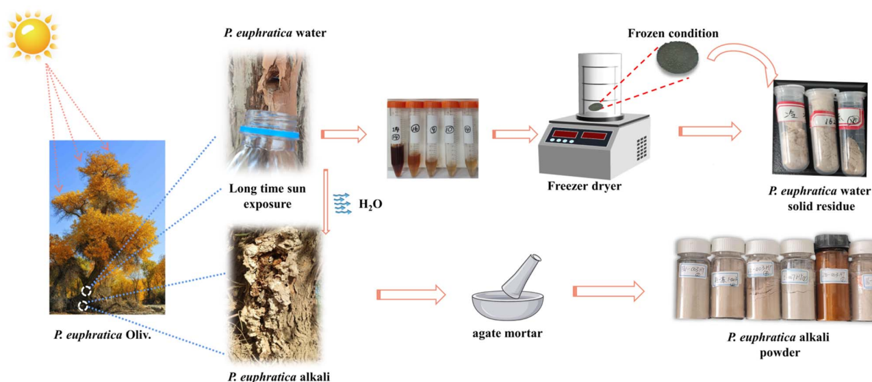
Fig. 2 Schematic diagram of PEW and PEA sample pretreatment.
