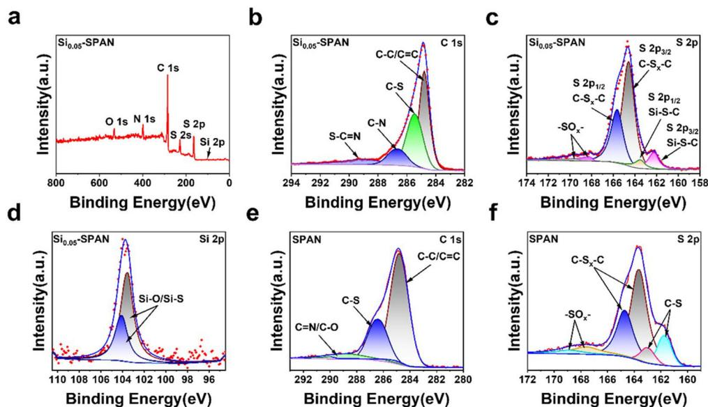
Fig. 3 (a) XPS survey spectra of the  $\text{Si}_{0.05}$ -SPAN sample. The elements Si, S, C, N and O are found in the sample; high-resolution XPS spectra of carbon (b), S 2p (c) and Si 2p (d) in  $\text{Si}_{0.05}$ -SPAN; and (e) high-resolution XPS of carbon (e) and S 2p (f) in SPAN.
