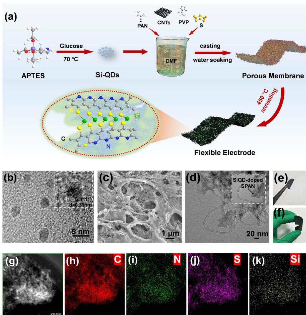
**Fig. 1** (a) Schematic diagram of the synthesis and structural evolution of the composite electrodes. (b)–(d) SEM and TEM images of the  $\text{Si}_{0.05}$ -SPAN composite electrode. (e and f) The mechanical test of the  $\text{Si}_{0.05}$ -SPAN composite electrode under different bending conditions. TEM dark field image (g) and the corresponding EDS elemental mappings of C, N, S and Si signals (h–k) for the  $\text{Si}_{0.05}$ -SPAN sample.
