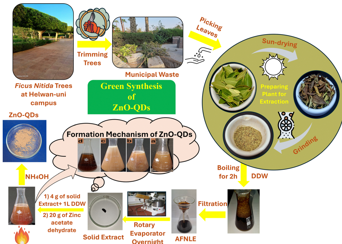
Fig. 1 Scheme of the green synthesis of ZnO-QDs using the aqueous Ficus nitida leaf extract.
